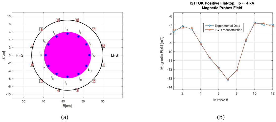
**Figure 4.** Figure 4a: ISTTOK Poloidal Cross Section with depiction of the radial and poloidal positions of the selected filaments for the plasma modelling and the magnetic probes. Figure 4b: comparison between magnetic probes measurements (blue line) and reconstructed values (orange line) during a plasma current positive Flat-top.
