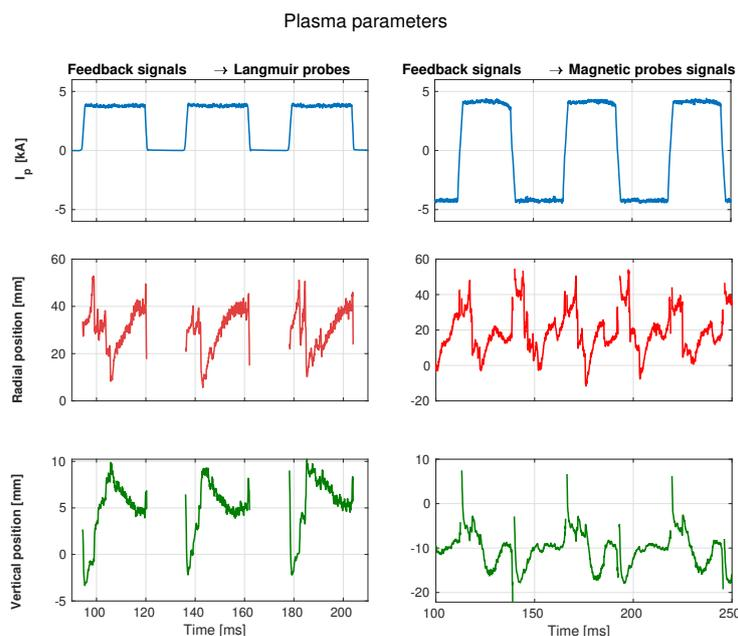
**Figure 9.** Real-time reconstruction of the vertical and horizontal current centroid position and plasma current assisted by the magnetic probes signal acquisition and post-processing of two plasma discharges. Left column shows the resulting signals when the discharge control feedback is performed using Langmuir probes and right column shows when using Magnetic probes signals. Negative plasma cycles are lost when using Langmuir probes signals.
