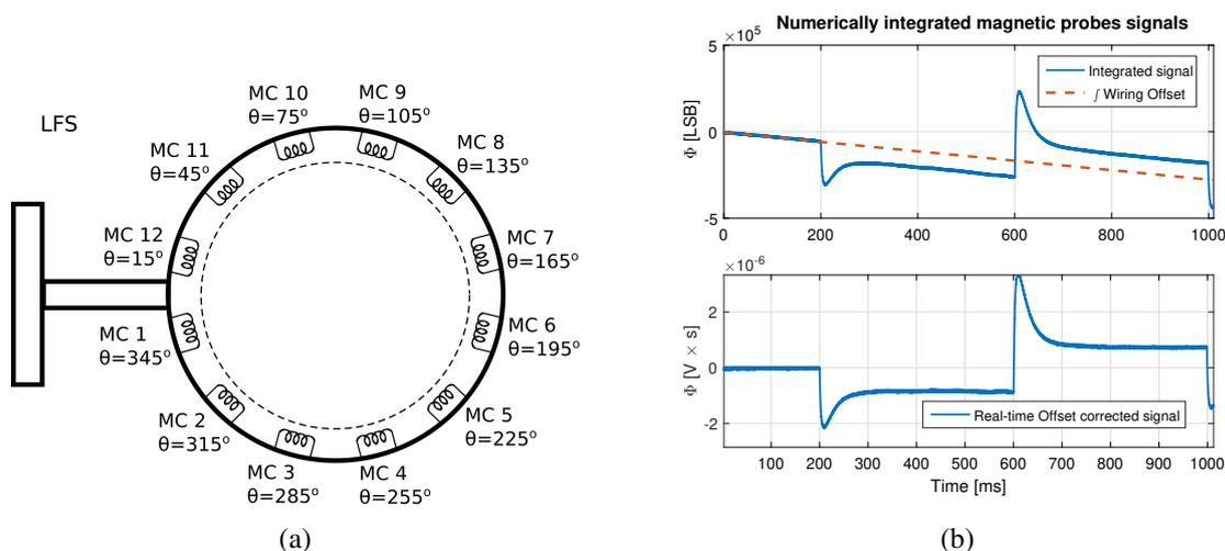
**Figure 1.** Figure 1a: set of 12 magnetic probes for the reconstruction of the plasma centroid position located along the poloidal direction at ISTTOK. Figure 1b: real-time subtraction from the integrated WO is performed on every MARTe cycle for each magnetic probe.
