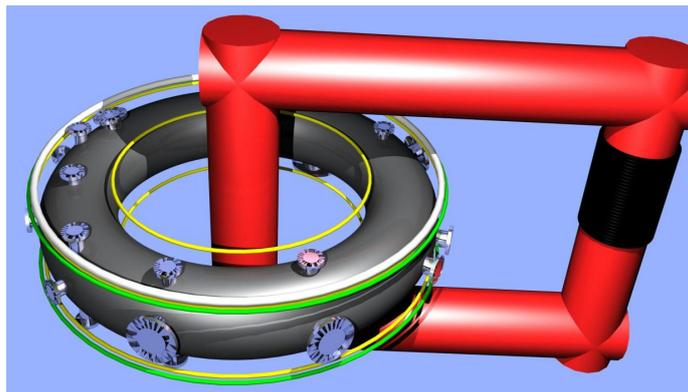
**Figure 2.** 3D scheme of the ISTTOK PF coils, vacuum chamber with ports, iron core and the former central solenoid (black color). Primary coils (white color) and horizontal coils (green color) are formed by 2 coils each one and located on the upper and lower LFS (Low Field Side) of tokamak. Vertical coils (yellow color) are formed by 4 coils, 2 are located on the upper and lower LFS and 2 in the upper and lower HFS (High Field Side). Figure 26 in section 1.5 of ref. [5].
